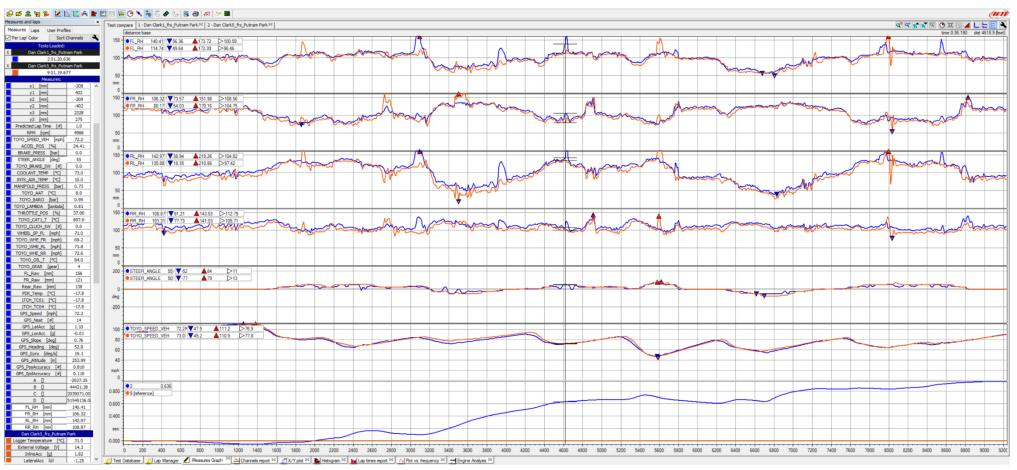
The orange lap is with Verus aero & UCW and blue is no aero. At the end of the straight, we are calculating around 420 lbs of downforce at 110 mph with wing angle of 1 degrees. The average downforce increased compared to no aero throughout the lap is 329 lbs.
