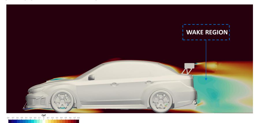
The CpT Plot shown above is used to visualize the wake region behind the car. The blue zone behind the vehicle is the wake and minimizing this as much as possible will reduce drag.
