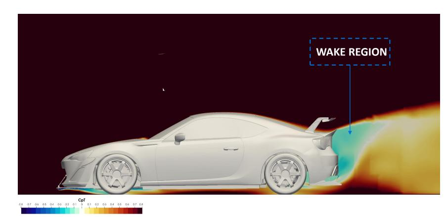
The CpT Plot shown above is used to visualize the wake region behind the car. The blue zone behind the vehicle is the wake and minimizing this as much as possible will reduce drag.
