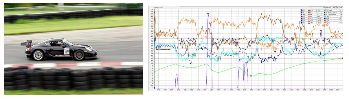
Ride heights correlated with downforce numbers when corrected for weight transfer and roll. We are still working on optimizing suspension setup to go with the added downforce.
