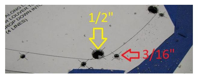
**2.19.** Using the template as a guide, cut out the section marked "cut out". The hood is steel and the paint is very easily burnt! This is normal and will be covered up with the flange of our hood louver.
