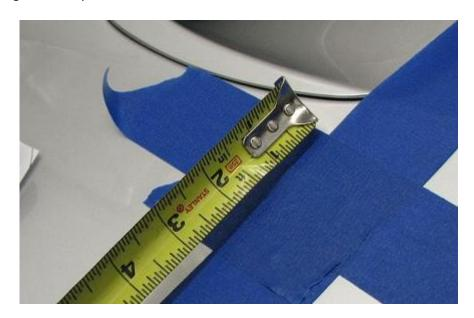
**2.12.** We have now found the location of the front, inside most hole location. This is positioned in the corner of the painters tape, shown below.
