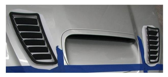
**2.16.** Center punch the center of each of the holes, as well as the holes on the inside of the template.
