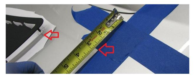
**2.13.** The louvers can still rotate since they are only placed in one spot right now. Ideally the louver outside curve lines up with the outside crease in the hood. We also measured towards the rear of the louver and got 5.5". **Ultimately, the big thing is that the sides are even and look the same.**
