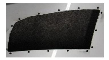
**2.26.** The hood's cuts **NEED** to be coated as the hood is some form of steel and it will rust in time. If you have touch up paint and want to coat the exposed edges, do so now and let it dry.
