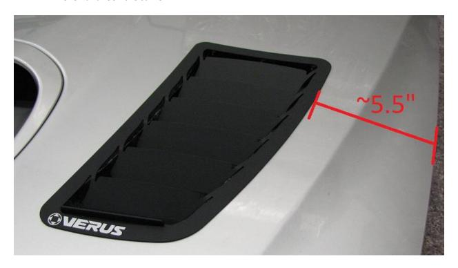
**2.14.** At this point, the louver placement is figured out and we can tape the templates to the hood. The biggest thing to ensure is that the templates stay flat to the hood to reduce discrepancies during drilling.
