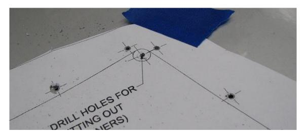
**2.18.** Enlarge the inside holes to  $\sim 1/2$ ". Enlarge the mounting holes to 3/16" initially.
