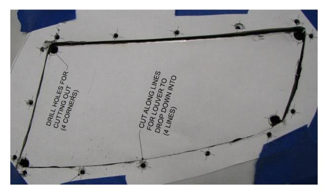
**2.20.** Remove the hood skin from the hood with needle nose pliers if necessary. The below image is what you will be left with.
