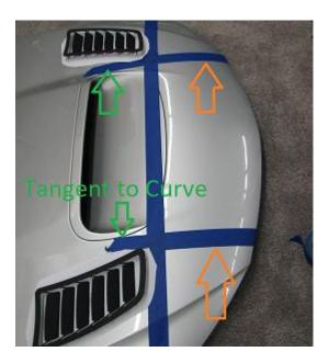
**2.11.** We then add another piece of tape, that has an edge dimension of 2.75" from the inside edge of the tape added in 2.10. This is shown below.
