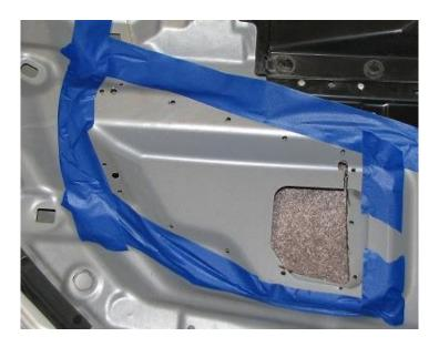
2.24. Using the cutoff wheel again, remove all of this material while giving ample room to tighten the nut on. This is shown below. \*Be sure that you do not cut through the hood's skin.\* This is likely the most difficult portion of the entire install! On areas close to the hood's skin, use light pressure and go slowly!
