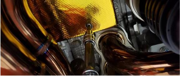
**3.12.** Install the small bracket supplied with the shield using the remaining supplied fasteners and long OE bolt into place. Do not tighten these bolts completely yet.
