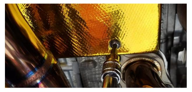
**3.15.** Ensure the shield is square with the timing cover and then finally tighten the fasteners on the outside bracket.
