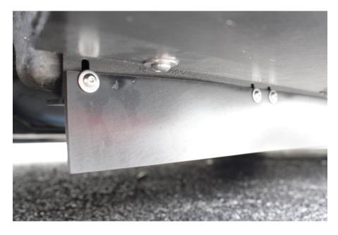
**2.13.** Install the (6) billet splitter mounts to the pinch welds, note that the front most mount has a different install detailed in 2.14. Use the M6 x 16mm long FHCS for the rear 5 mounts on each side. Bolt through the mount, through the pinch weld, and then a nut on the inside. Do not fully tighten at this time.
