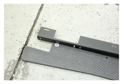
**2.12.** Next, we install the two-piece side skirts. Use the M4 BHCS, washers, and the lock nuts for these. The front and rear sections are NOT identical.
