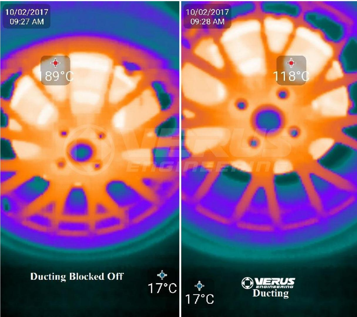
Photo was taken after a short cool down driving at a moderate pace. Similar to that of a cool-down lap, no hard braking was used.
