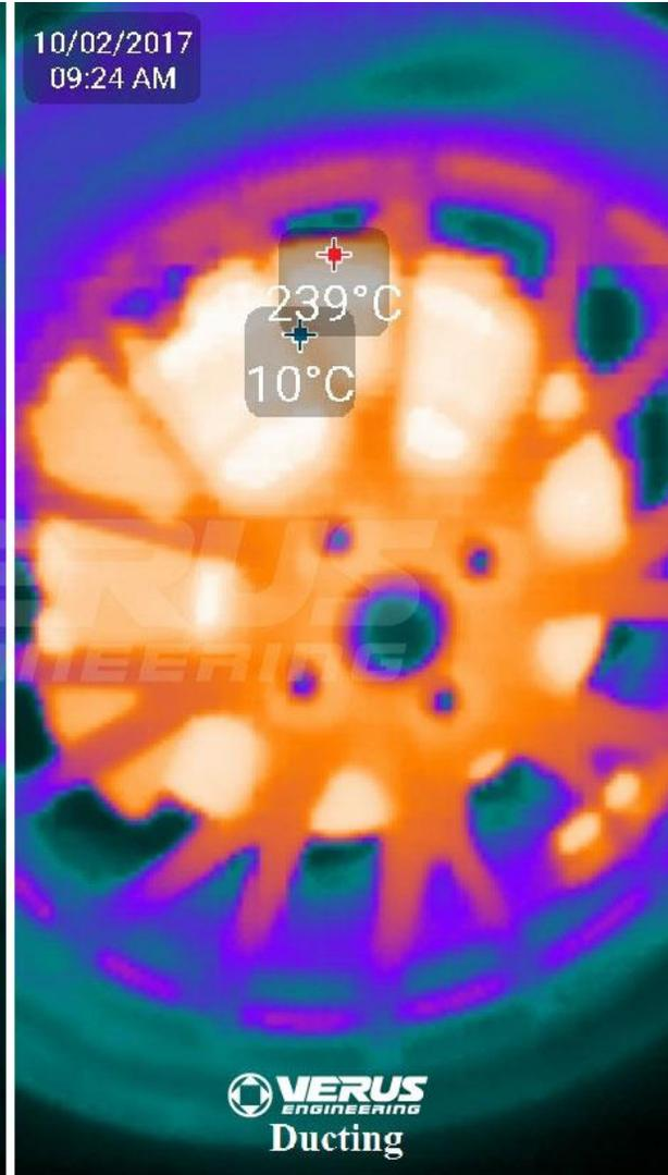
Photo was taken directly after testing a hard braking event from 60MPH to 0.
