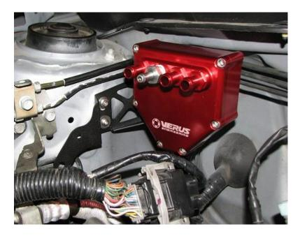
**2.19.** Install the OEM bracket removed in 2.16 and install this on the bolt locations located on the left of the bracket. Use the M6x1.0 x 12mm BHCS, fender washers, and serrated nuts to install this.
