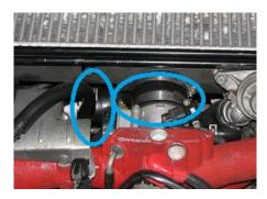
**2.6.** We can remove the charge cooler by removing the (2) 12mm bolts holding the cooler to the cooler brackets, these are circled below in orange.
