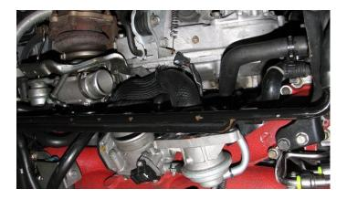
**2.8.** We can now remove the hose that goes from the PCV valve to the intake manifold. This is located directly below the throttle body, circled below in yellow.
