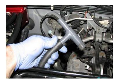
**4.3.** Install the T fitting into the 3/4" hose into the block port we installed at 4.1.
