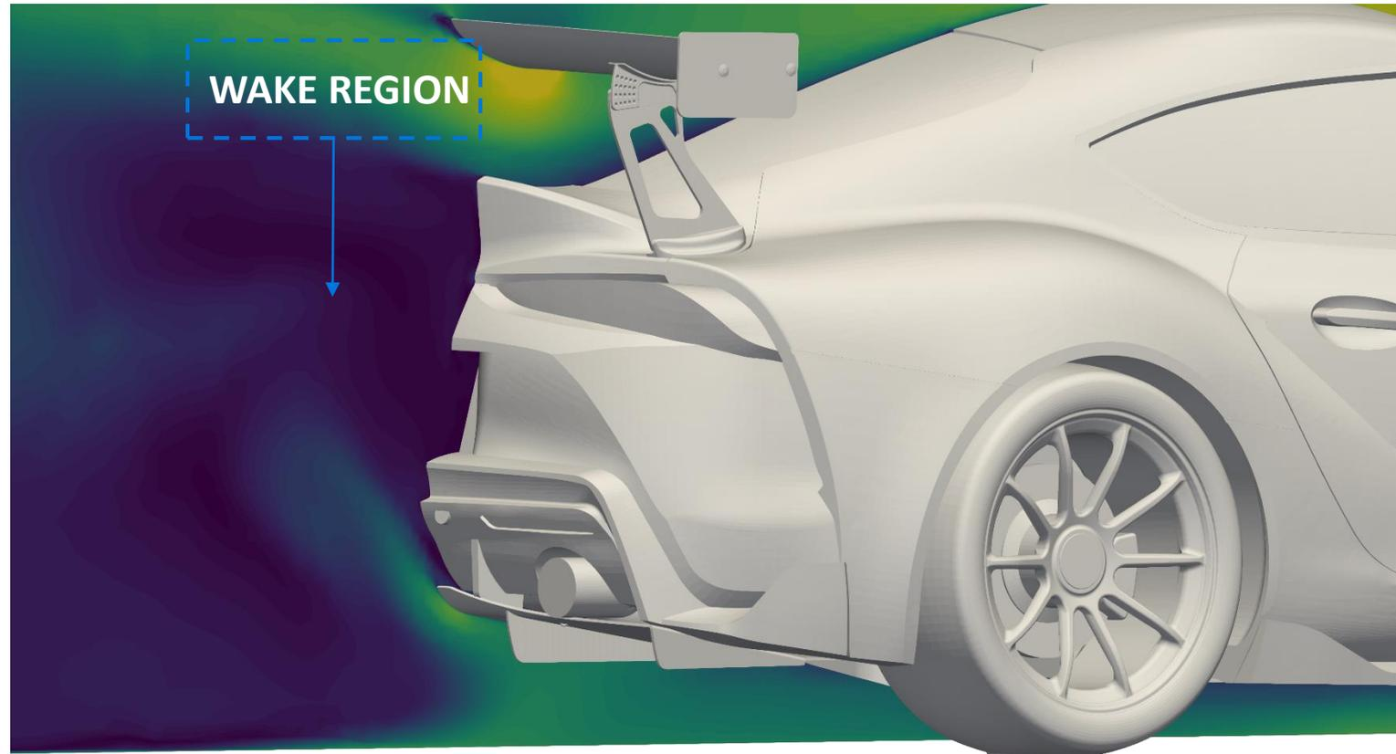
The Velocity Plot shown above is used to visualize the wake region behind the car. The blue zone behind the vehicle is the wake and minimizing this as much as possible will reduce drag.
