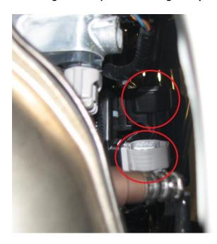
7. You will now need to remove the exhaust manifold. Use a deep 14mm socket to remove the (8) exhaust manifold nuts circled in red below. Note: The manifold may take some effort to get off of the studs.
