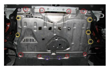
**4.** Once the engine shield is removed, use the 17mm socket to drain the oil from the OEM pan.
