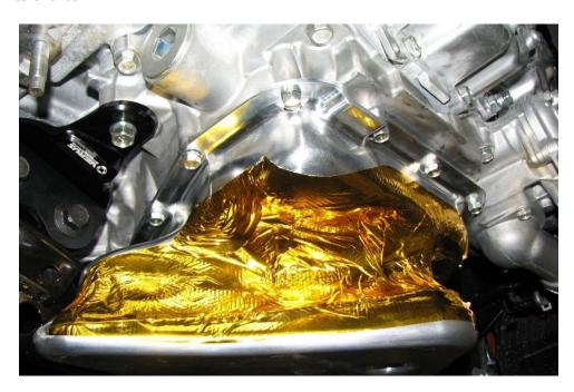
**22.** You may have issues installing the factory hardware in the rear middle of the pan. If you do, please use the M6 x 12mm long SHCS with lock washer provided in the kit and install using a 5mm allen wrench.
