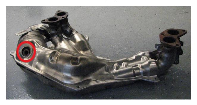
**9.** Remove the (7) bolts using a rachet or impact driver with a 10mm socket. Remove the top and bottom heat shield and set them aside, they will not be reinstalled.
