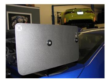
**23.** For the best results, the endplates should be installed with the top edge parallel to the ground. You can do this by utilizing a household bubble level as shown below.
