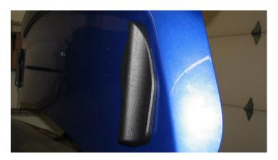
**17.** Close the trunk and install the uprights with the (2 per side) M6 16mm long BHCS and (2 per side) 12mm OD washers. Torque to 6 ft-lbs.
