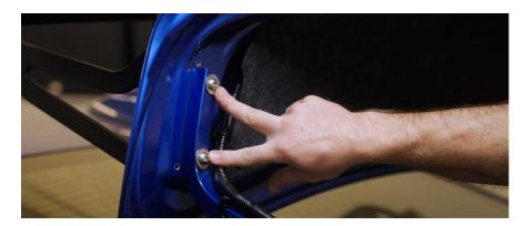
7. Use a 5/16" drill bit, drill straight through the (4) trunk mounting holes to get rid of the threads. The OEM trunk mounting holes are used as guides for drilling these holes. **Note:**Once you get through the threaded portion, keep drilling through the top skin on the trunk.
