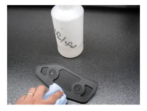
10. Peel back the white backing and place the 3M VHB on the trunk mounts.
