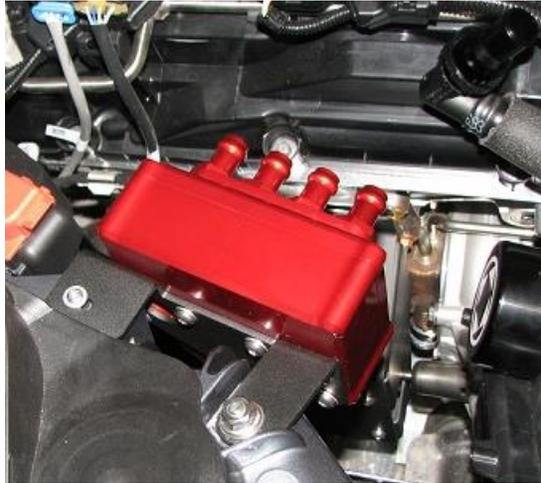
**2.10.** Tighten the T20 bolt to snug, and the 13mm bolt to factory spec, 21 ft-lbs + 90 degree turn.
