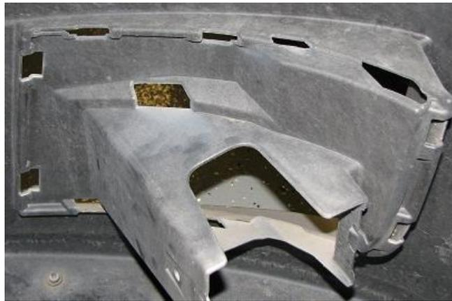
2.22. On the outside tab, we will drill a hole for the bracket to bolt to. We use calipers or a tape measure to mark this point. 14mm, or 0.55", should be marked as shown below.
