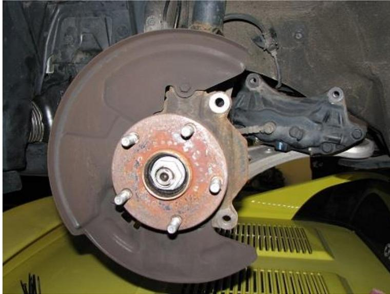
2.8. Remove the OEM backing plate by unbolting the (3) 12mm bolts circled in yellow below.
