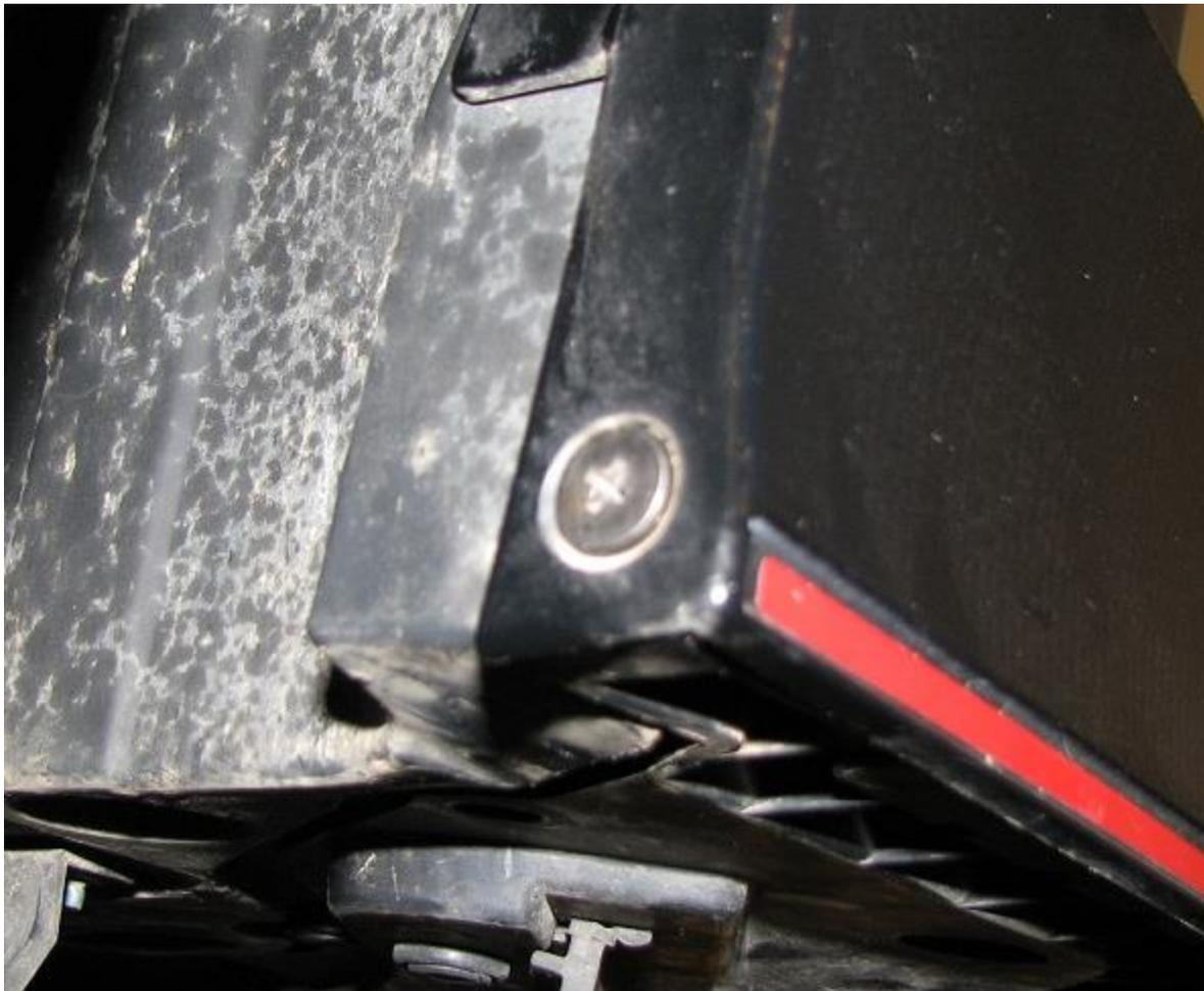
2.7. Remove the bolts circled below, one is an allen bolt, the other is a standard hex head bolt.
