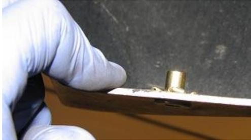
**2.13.** With the rivet nut installed, we can install the rear bracket.
