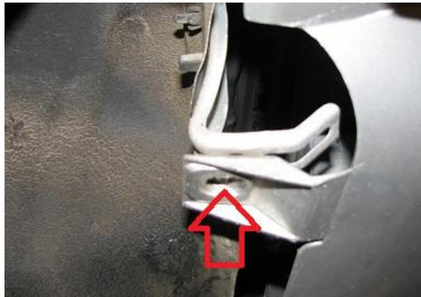
**2.15.** Install the rear bracket as shown below with a 16mm long M6 BHCS, washer, and serrated nut.
