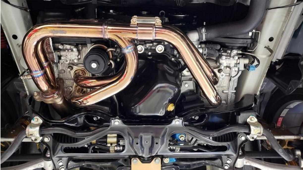
3.6. Remove the factory AVCS cover by removing the 10mm bolt (yellow arrow) and unclipping the plastic clip towards the back (red arrow).
