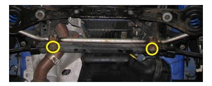
**3.2.** Install the front brackets as shown below. The flange should face forward and be near horizontal when installed.
