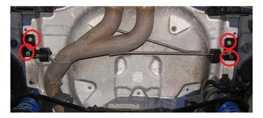
**2.6.** To install the brackets, the bottom surface should slant upward towards the rear with the flanges pointed towards the center of the vehicle. They are side specific.
