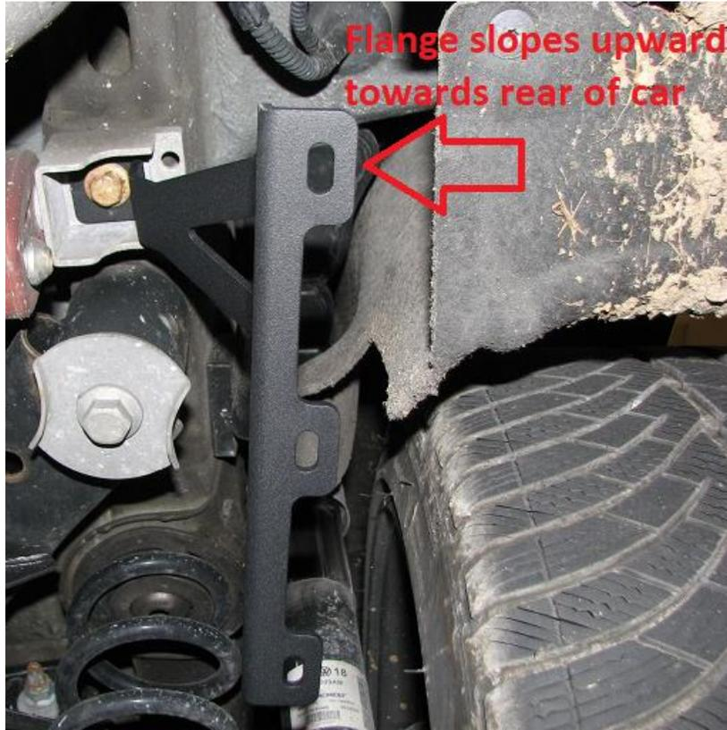
2.9. Finally, we move to the rear brackets. Remove the bolt with an appropriate bit.
