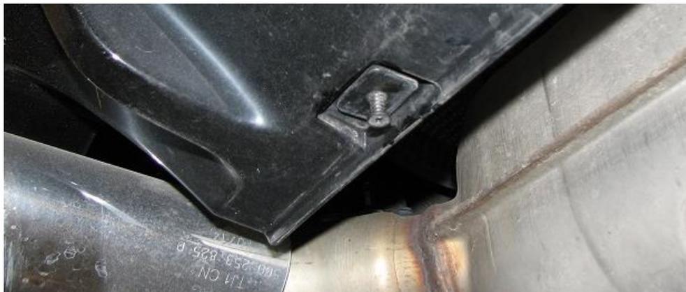
2.10. Pull down on the bumper to remove the plastic clip completely.
