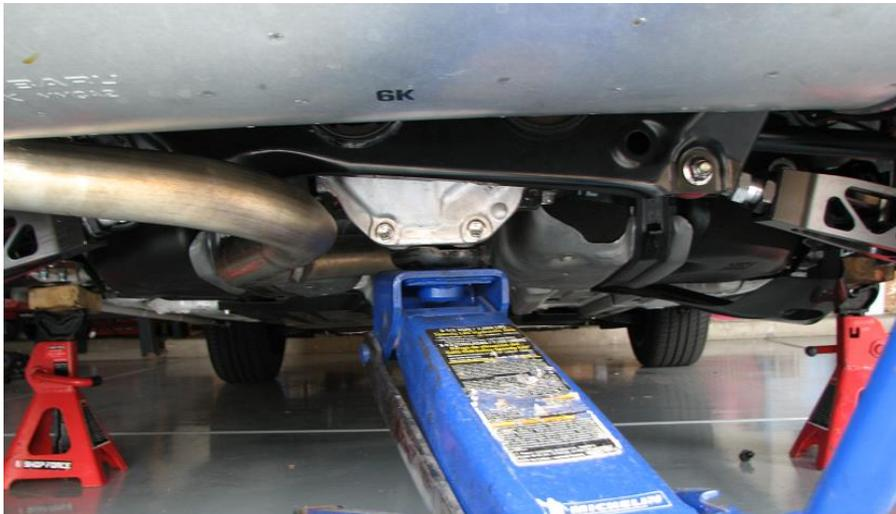
2.3. Remove the exhaust from the front pipe backward. Depending on your exhaust, this will be 12mm or 14mm bolts on the front and whatever is on the rear.
