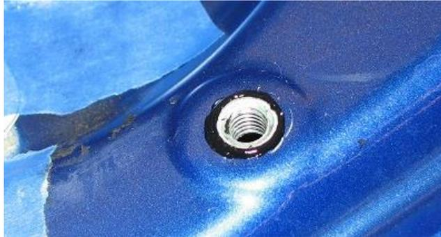
2.16. With the rivet nut installed, and the holes drilled to 9/32", we can flip the trunk over and start working from the top side of the trunk.
