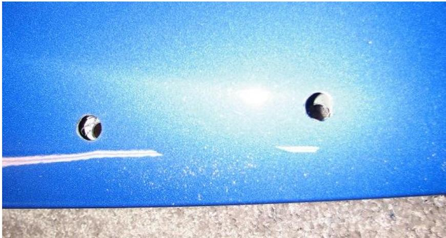
2.18. With the holes slightly larger, we can now use a carbide bit and grinder to open these holes up larger. **You will want the holes to be slightly larger than bungs on the mount.**
