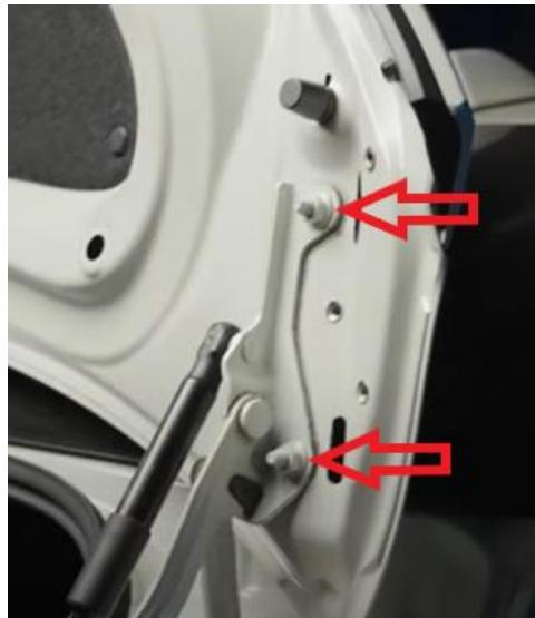
5. With the mounting nuts removed, install the support bracket as shown below.
