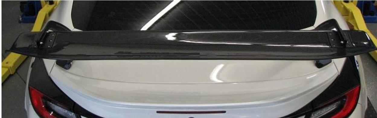
**21.** Use the diagrams below to adjust your desired “Angle of Attack” for your wing blade before proceeding. **Note: We recommend starting with a higher Angle of Attack and slowly decreasing it to balance the vehicle to your liking.**
