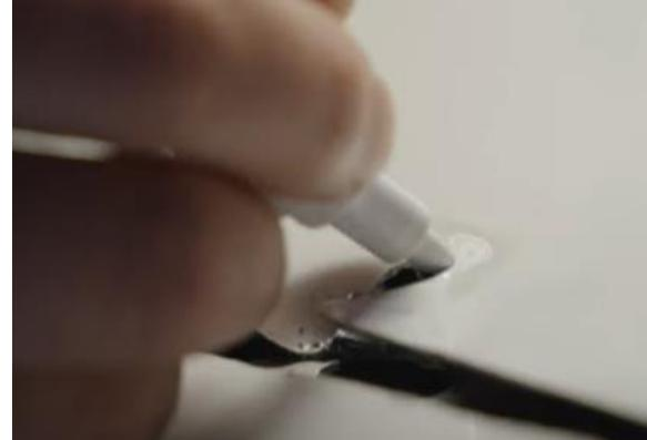
12. It is now time to prepare the trunk mounts. Clean the groove in the trunk mount with 50/50 mix of isopropyl alcohol and water. This is where we will install our die cut 3M tape.
