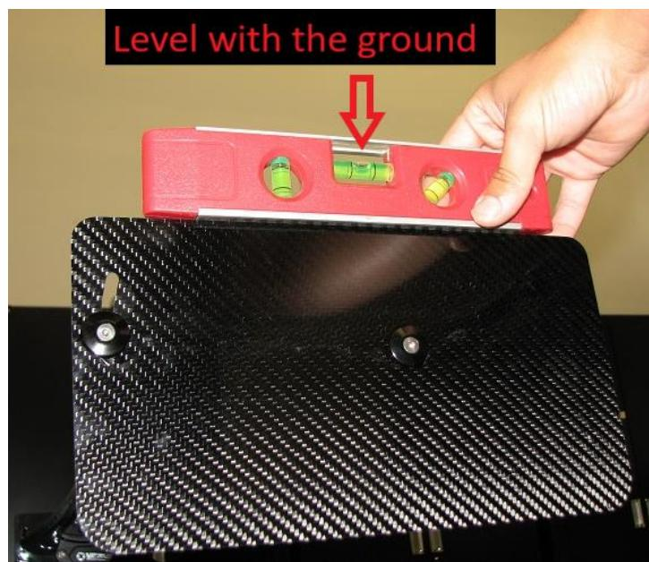
**28.** Once the endplate is level, tighten down the endplate fasteners. **Note: The endplate fasteners only need to be tightened a few in. lbs.**
