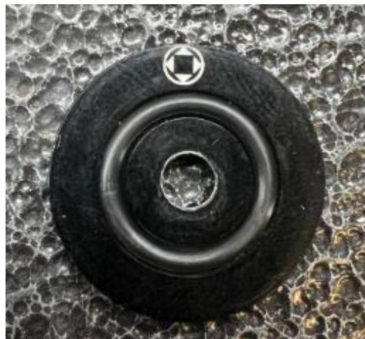
25. Then place it flat against the endplate so that the M4 FHCS can pass through the mounting hole. **Note: Be sure that the O-ring is lying flat inside the groove before proceeding.**
