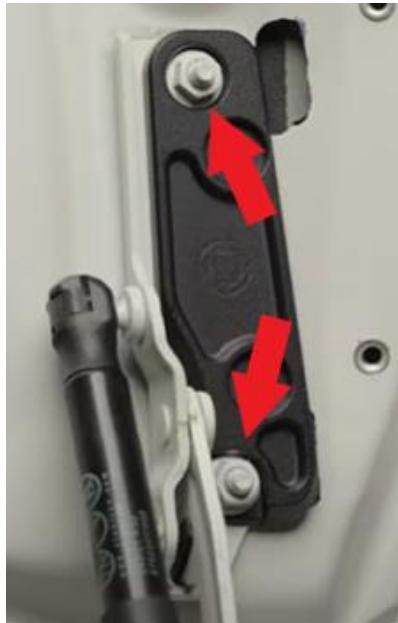
7. At this time, you may either mark your desired drill locations and then remove the trunk bracket to drill the holes. Or, you can use the mount as a drill template and drill through the holes on the bracket as we have done below. **Note: These holes will be drilled through all layers of the trunk, including the outer skin. That being said, drill as perpendicular to the mounting bracket surface as possible.**
