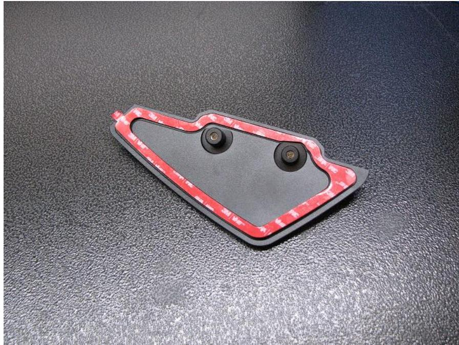
**14.** Clean the trunk surface where the mount is going to sit with a microfiber and 50/50 alcohol water mix. Then, peel back the red tape layer and place the mount onto the trunk surface.
