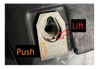
16. Install the clip-on nuts (removed in the previous step) onto the engine splash shield.
