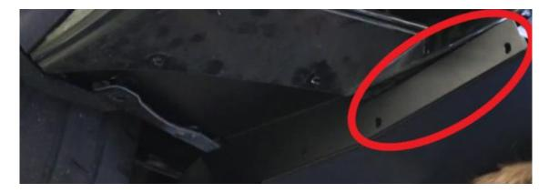
27. Repeat installation on the remaining side. Note: The fully installed side plate should sit flush and flat with the fender liner as shown in the image below.
