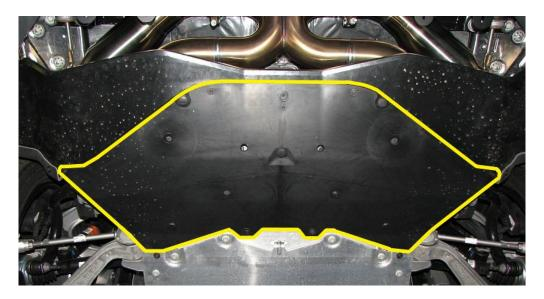
4. To remove the first splash shield, there will be (11, circled in red) 7mm head screws and (1, circled in yellow) plastic push clip. Note: This splash shield will not be reused with the diffuser. However, we will need to use (2) clip-on nuts from this so keep it close for now.
