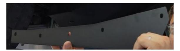
33. Place the diffuser strake between the main and side plate. Use the M6 16mm long BHCS stainless or black oxide with washer, and M6 serrated nut to fasten all (3) layers together.
