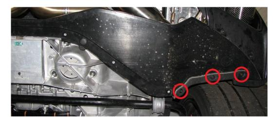
7. Next, remove (4 total) T15 screws (passenger side circled in orange below).
