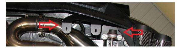
**14.** We now need to shift back to the splash shield we removed in **Step 4**. The front clip-on nuts will need to be removed and reused on the car.
