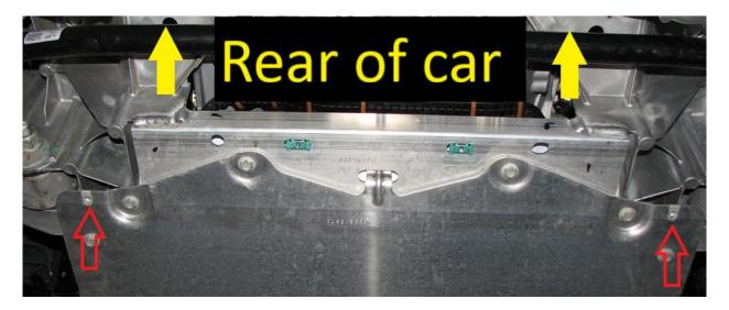
17. Test fit the main diffuser element at this time. Use this step to adjust the fitment of brackets previously installed in Steps 11 and 12. Note: We used the center 7mm head screw along with (2) front 7mm screws to gauge fitment.
