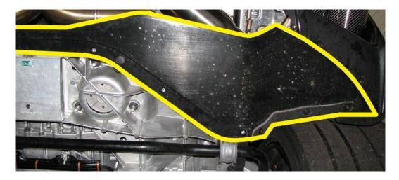
**6.** Remove the (6 total) 7mm head screws (passenger side circled in red below) for the splash shield first.
