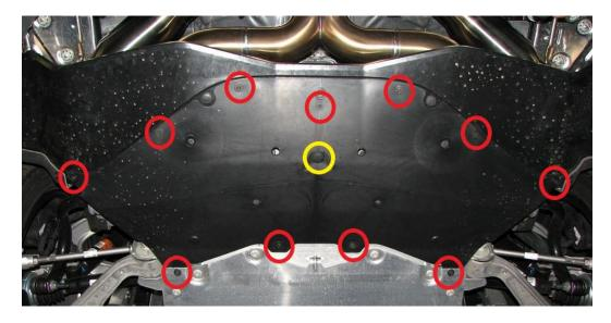
5. With this shield out of the way, we can remove the remaining splash shield that runs the width of the car. The passenger side of this splash shield is outlined below. Note: This splash shield will not be reused with our new diffuser. Safely store or discard the shield at this time.
