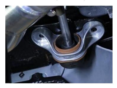
12. Install one of the diffuser brackets by sandwiching it between the body and exhaust hanger. Loosely reinstall the 13 mm head bolts. Note: The Passenger side is shown below. Notice the Verus logo is legible through the bumper grille.
