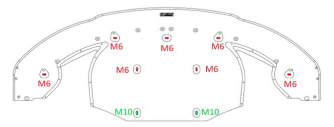
**18.** Adjust your splitter rod ends so that the splitter sits level side to side as well as front to back.
