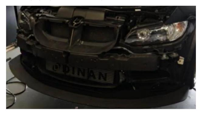
**19.** Once your splitter is leveled to your liking, loosely install the air dam using the M6 BHCS 16mm long, M6 18mm OD washers, and M6 Serrated nuts.
