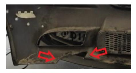
**24.** Once the bumper is trimmed, make sure all of your clevis and support rod connections are tight. Then, reinstall the front bumper. **Note:** We were able to reinstall the front bumper with the splitter and air dam still installed.
