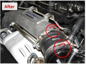
13. Connect 30" of hose to this reducer and route it as shown below. Note: This routing is just a recommendation. You are able to run the hose however you see fit.
