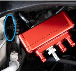
**25.** With the AOS mounted, we will return to the metal PCV pipe we connected earlier and pinch off the coolant lines.
