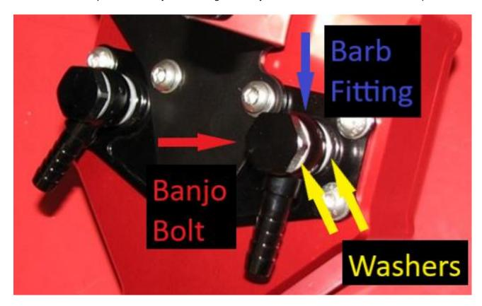
**21.** Attach 15" of hose to the outer/passenger hose and 33" to the inner/driver hose. Tighten hoses to banjo barb fittings with hose clamps.
