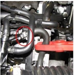
**39.** Route the coolant hoses over the engine (as shown below) and connect them together using a 5/16" barb connector and (2) hose clamps.
