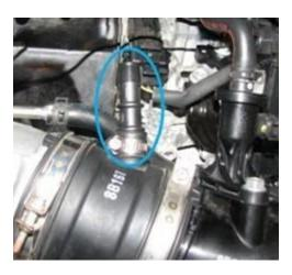
**12.** It is now necessary to rotate the intake coupler. The coupler should be rotated about 1/2" towards the engine as shown below.
