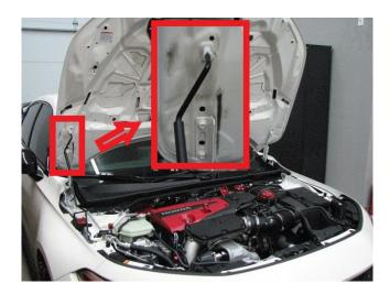
3. Once the hood is opened, take off the engine cover by removing the (5) 10mm bolts.
