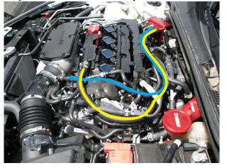
**16.** With the longest hoses routed, we can now prepare the AOS to be installed. **Note: If you are not installing the coolant add-on kit, skip to Step 34.**
