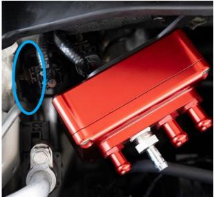
**37.** With the AOS mounted, we will return to the metal PCV pipe we connected earlier and pinch off the coolant lines.
