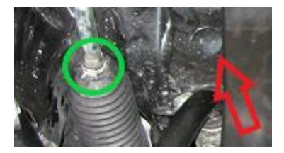
**38.** Check to make sure all of your clamps and zip ties are tight. **Note: Make sure the clamps** on your tie rod ends are facing down and not contacting the hoses as circled in the image above.
