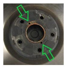
**27.** You can now take both factory dust shields off by removing the (3 per shield) 12mm head bolts.
