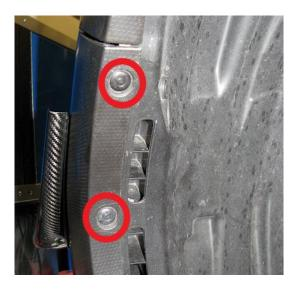
13. The remaining clips holding the bumper on are hidden. You will find the first ones where the bumper and fender meet at the wheel well. Grab both layers of the bumper (bumper and fender garnish) and pull outwards (towards you). This will release (5 per side) clips holding the bumper to the fenders.
