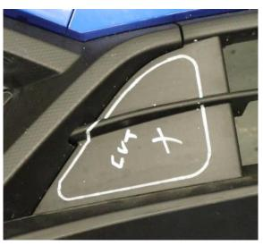
18. Once the line is traced, remove the template and use a cutoff wheel or reciprocating saw to cut along the line. Note: After cutting along the line provided by the template, small amounts of trimming will still be needed. We trimmed the outer grille line further back (shown with green arrow below) as well as angling the cut for the inner grille line (shown with yellow arrow below).
