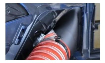
**31.** With the help of a friend, reinstall the front bumper. The cooling duct hoses will need guided in as the bumper goes on. The driver side will go between the exhaust and the washer fluid reservoir. The passenger side routes under the intake tube. Both sides will enter the wheel well next to the subframe mounting brackets. **Note: Below are images of hose routing.**
