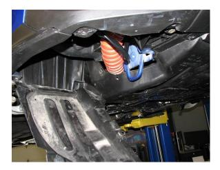
**9.** You should now be able to see the backside of the fog lights (if equipped). Unplug both fog light connectors.
