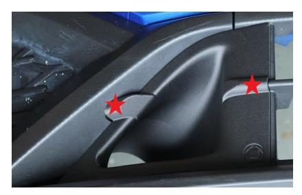
**22.** Now that the ducts are fitted, install the ducts onto the bumper. Once the tube section is through, angle the corners into place (refer to image below).
