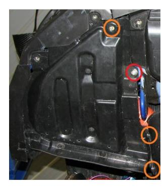
8. Having freed up the front section of both fender liners, pull them down and back. Note: The hose should not be installed right now (as shown below), but this is where the hose will be installed.
