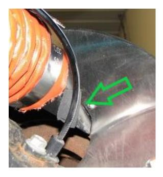
**30.** We should now be ready to attach our 2.5" high temp hose to our bumper with the provided 2.5" hose clamps. **Note: Connect both hoses to the ducts and give them a pull, if they do not slide off then they are tight enough. Over-tightening can damage the clamp or duct.**
