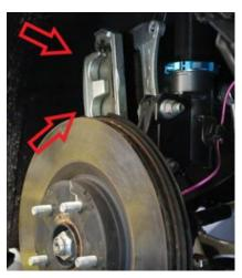
26. With the calipers out of the way, remove the rotors. Note: If you are reusing your rotors, either use a plastic dead blow hammer or the M8x1.25 threads on the face of the rotor hub provided by Subaru.
