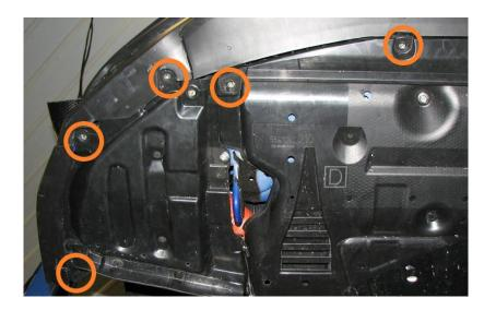
7. While still under the car, we need to loosen the front section of both wheel wells. This is done by removing (3 per side) center-pull type clips circled in orange below (there will only be (2) if you have our front splitter) and (1) 10mm screw that is circled in red below.
