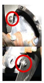
**29.** Attach the 1" section of adhesive foam tape between the ABS sensor wire and the duct. You can place this on the duct or wrap it around the ABS wire. **Note: This is to protect the harness from rubbing on the duct.**
