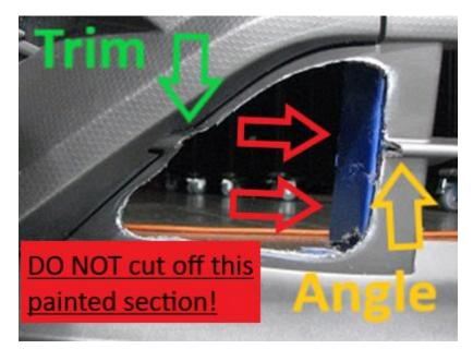
19. Now that the main hole has been cut out and trimmed, cut out the slot for the duct mounting tab. Note: This can be done with any cutting device. We made our slot by drilling a series of 1/8" holes and "connecting the dots".
