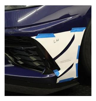
2.7. Before installing the dive plane, place each dive plane in the correct location. Ensure the template is properly installed and that when you install the units in their final location, there are little to no gaps between dive plane and bumper. Note: The larger dive plane is the lower and the smaller dive plane is the upper.
