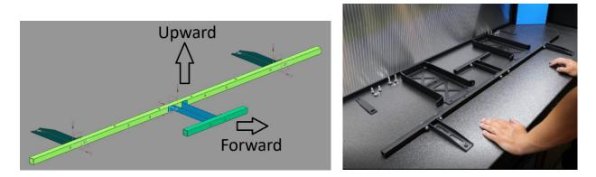
**2.43.** The support bracket assembly can be installed on the car now. Each upright will have (4) screws attaching it to the support assembly. (2) of the bolts going up and down and (2) going front to back. The outer screw for each upright will get the small bracket with 1 bent end. Refer to image below for visual reference of assembly installed on the car, side brackets are circled in yellow.
