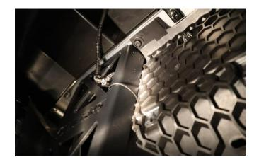
**2.26.** It is now necessary to trim the splash shield we removed earlier. Trace the inner rectangle and cut the inner section of the rectangles out. We used a reciprocating saw for these cuts. The templates and finished product are shown below.
