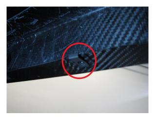
2.37. Install the preassembled air dam while making sure it sits flush and even with the bumper. Note: The fasteners closest to the wheel wells are a tight fit. We used a screw driver style T15 to tighten these.
