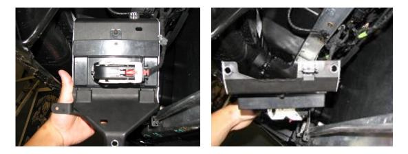
**2.18.** Reinstall the bracket and proceed with installation. We recommend zip tying the wire harness up out of the way.
