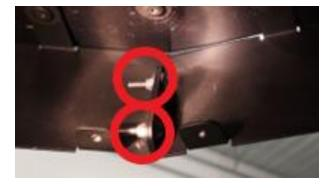
**2.34.** Not all the hardware removed from the OEM lip is needed to attach the new air dam. Please reinstall all the hardware not used for the air dam.
