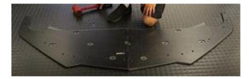
**2.5.** Once the halves are put together nicely, we need to install (2) 20mm long M4 BHCS that pass through the center of the zipper fit. Tighten down on the backside with a washer and nyloc nut.
