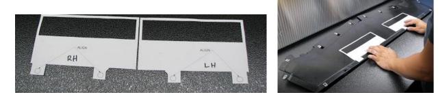
**2.27.** The newly cut splash shield can be reinstalled. The previously installed upright brackets should pass through the openings that were cut out.
