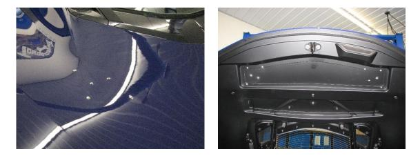
**2.7.** Now that our holes are drilled, we need to check that our upper mounting studs line up. Test fit both mounts, they are directional and will only fit one way. If a stud has trouble going through all the way, use your drill bit again to open up the holes. Repeat until upper mount will sit flat on the trunk. **Note: Do NOT remove red backing tape yet, this is only a test fit.**
