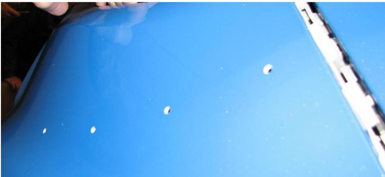
2.13. With the nuts and washers on the rear side of the bumper, you can tighten the bolts on the dive planes. We found tightening the nuts from the back side with a ratchet and socket to be easiest.
