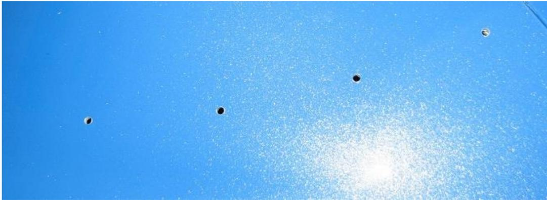
2.10. Using the countersink, clean the holes from any burrs from drilling.
