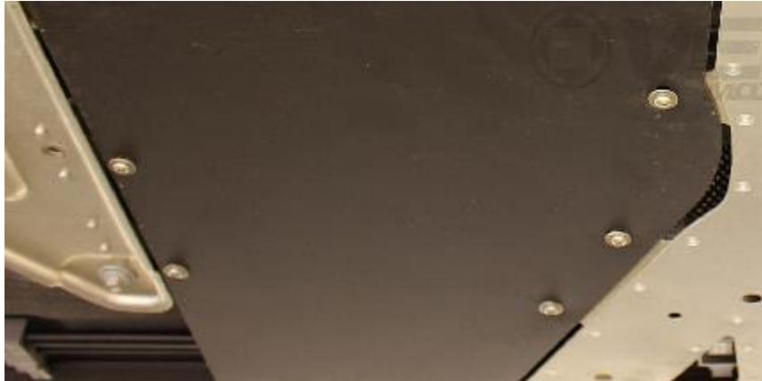
**3.2.** Using a sharpie or paint marker, mark the center of the (3) slots on the rear panel, located below in blue.
