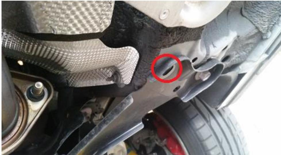
**2.8.** We can now install the front panel. First bolt the 17mm bolt with the panel now on top of it. Tighten this to 48 ft-lbs.
