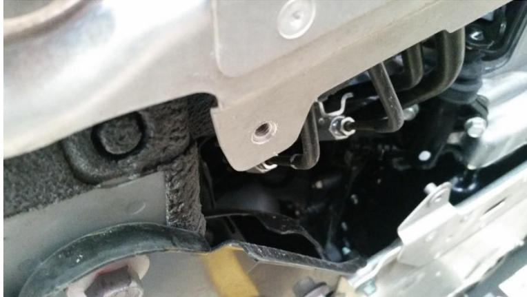
**2.7.** Remove the large sub frame bolt with 17mm socket.
