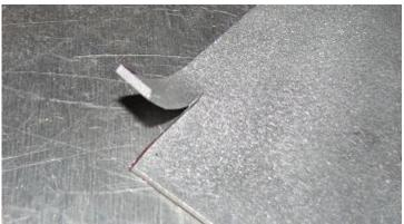
**6.10.** Using the 90 degree angle grinder and sheet metal finisher, clean up the cuts so that the edges are nicely finished.
