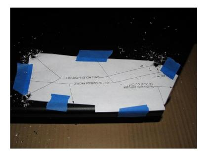
**6.7.** Using the stepped drill bit, drill through the diffuser completely and pull off the template. Countersink the holes. Using the template and blue tape, map out how you will cut the diffuser.
