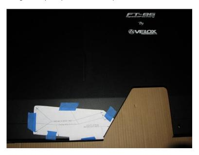
**6.5.** Using the hammer, a center punch, and something beneath the diffuser for support (2x4s work well), center punch the (3) holes marked on the template.
