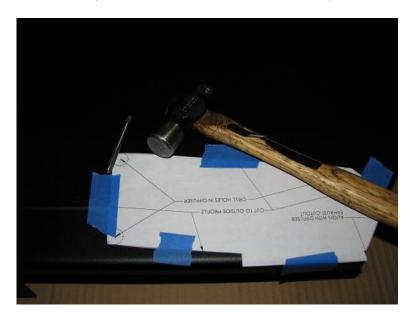
**6.6.** With these holes center punched, use the pilot drill bit to get the holes started.
