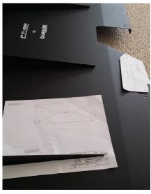
**6.4.** Using blue tape, tape the below template onto the bottom side of the diffuser as shown below.
