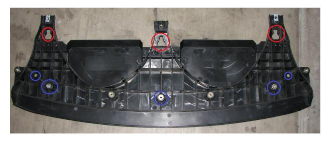
2.6. Next step is removing the front bumper. To remove the front bumper, remove the strip of 10mm bolts and plastic push pins across the top of the front bumper under the hood.
