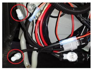
**3.13.** Next, let's wire the positive side of the relays. Run the two yellow wires to the positive terminal of the battery and wire in the 30 amp fuses included in the relay kit.
