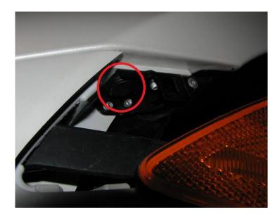
**2.10.** Remove the intake and intake filter so that we have room to remove the radiator later. Below is a photo with the front bumper removed as well as all intake related components.
