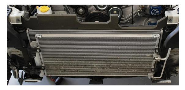
**2.15.** Remove the (4) 10mm bolts from the condenser to the radiator, circled in blue below.
