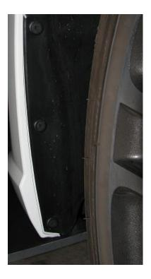
**2.8.** The turn signal has to be removed to expose the final plastic push pin and then the front bumper will come off. There is a metal tab that needs to be push towards the \*front\* of the car. The arrow in the picture shows this well. I used a flat head screwdriver to push this forward and then gently pried the signal away from the car.
