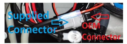
**3.8.** With the OEM connector from the fan shroud we de-pinned in step 2.24, plug in the two remaining flying leads we supply in the kit. The other option, if you did not want to de-pin the connector, is to cut the wires with about 12" of lead remaining. Below is a de-pinned OEM connector with OEM flying leads in it.
