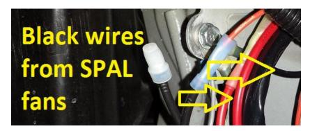
**3.17.** The fans are wired up now. You can test your wiring a number of ways **once you connect the battery again**. You can test by powering the signal wire of the relay, this should kick each fan on. Remember to not touch the "hot" power to any grounds on the car.
