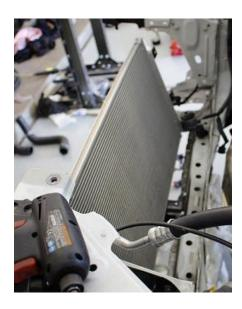
**2.21.** With the radiator out of the car, we can get the new Verus Engineering radiator ready for install! We start by uninstalling the overflow from the OEM radiator by removing the (2) 10mm bolts circled below in yellow. The overflow has already been removed in the below photo.
