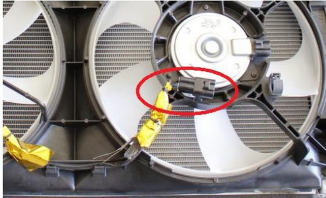
**2.24.** To de-pin the connector. Depinning the connector can be a bit frustrating and is a two-step process. You must first release the pin guard. Pull this guard piece out of the connector to expose the pins, then using a de-pin tool or paper clip, remove the wires from the connector as shown below.
