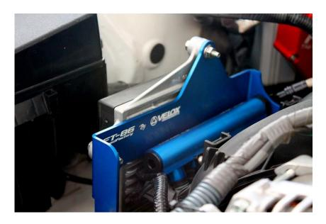
2.9. Install the small wire clip into the bracket where the small round hole. This is circled below in yellow.
