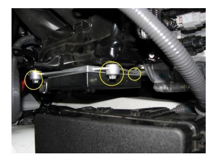
2.6. Remove the fuel rail cover by taking the two 12mm bolts off (circled in blue). There are various electrical pieces that are connected to the cover, remove these as well.
