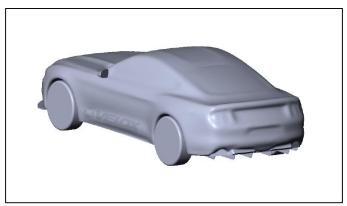
Figure 2.1.2: Geometry Simplifications – Rear ISO
