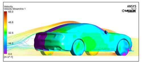
Figure 5.7.4: Streamlines Off the Diffuser
