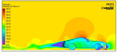
Figure 5.4.1: Velocity Plot Symmetry Plane
