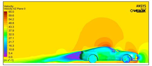
Figure 1.3.3: Stock Mustang – Velocity Cut Plane
