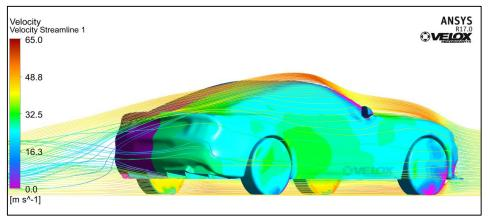
Figure 5.7.5: Streamlines Off the Diffuser
