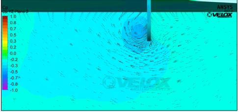
Figure 1.3.3: Vortex on the Velox Diffuser Strake
