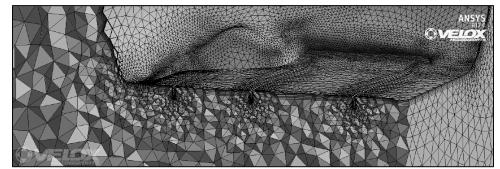
Figure 2.4.4: Mesh Section View at Diffuser
