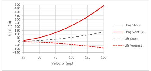
Figure 5.2.1: Aerodynamic Forces at Speed
