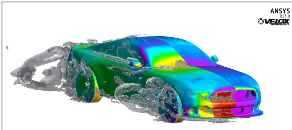
Figure 5.7.2: Q-Criterion Displays Vortices Forming on Splitter
