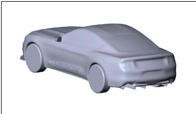
Figure 2.1.2: Geometry Simplifications – Rear ISO
