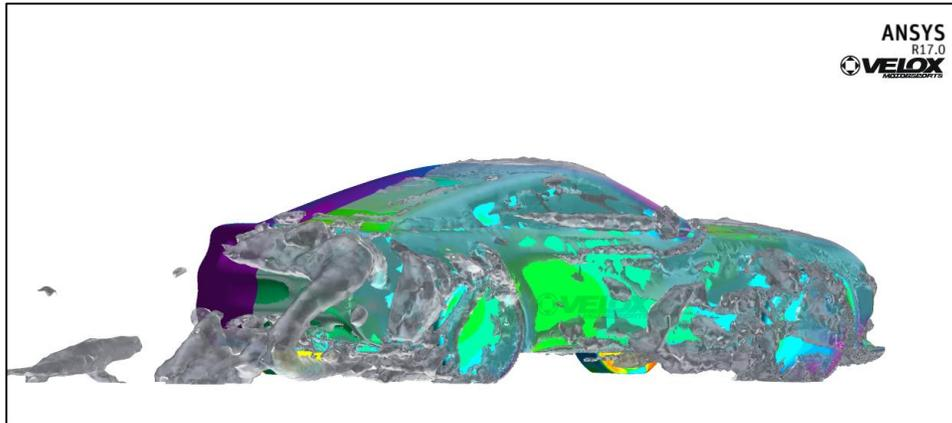
Figure 5.7.1: Q-Criterion Displays Vortices off the Mustang
