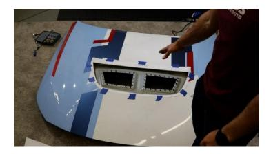
**2.7.** Mark the cut area with painter's tape around the structure as shown below. We are using the raised edge to keep the cut off wheel away from the hood skin. A photo of what this should look like is below.
