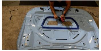
**2.9.** Remove the under-hood structure you just cut out. You can also remove the painter's tape at this point on the bottom side of the hood.
