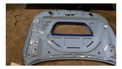
**2.10.** Flip the hood back over and test fit the hood louver before the template is removed. We do this to ensure the hood louver will sit flush with the hood. If it does not, make the necessary cuts to ensure it does sit flush.
