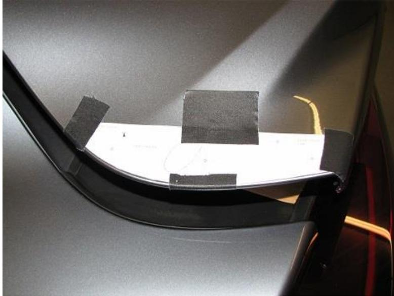
2.5. With the template taped in place, place the trunk mount on the trunk with the holes located where the paper template holes are. Ensure that the trunk mount appears to sit on the trunk well and that the holes line up. Ensure that the trunk mount sits cleanly on the outside edge of the trunk. This is a sanity check before drilling holes in your trunk.
