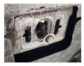
**2.5.** Install the supplied o-ring into the new anodized jack puck. Using a small amount of Sil-Glyde will help the o-ring stay put inside the jack puck.
