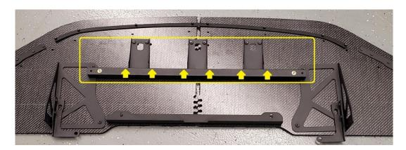
**2.29.** Bolt the cross brace to the main splitter brackets using the holes and orientation that is shown below. Use 40mm long BHCS, 12mm washers, and M6 serrated flange nuts. Torque to 6 ft-lbs. The washer should be under the bolt head, and facing the ground.
