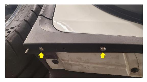
**2.41.** Slide the center air dam bracket into place so that it lines up with the remaining air dam holes that were drilled in **2.3.2**. Once the holes line up, install the supplied m4 studs into **every other hole.** This applies to the remaining holes in the side air dam brackets as well. These studs will be used to locate the air dam bracket correctly into the splitter.
