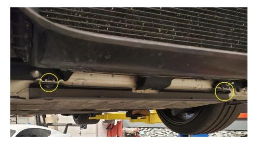
**2.26.** Bolt the side chassis brackets to the main splitter brackets with 20mm long M6 button head cap screws, and 12mm O.D. washers. Torque to 6 ft-lbs.
