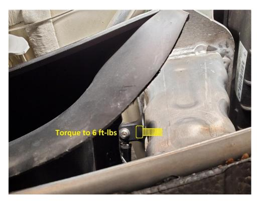
**2.34.** Also torque the clevis on the cross brace to 6 ft-lbs.
