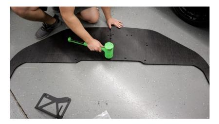
**2.3.1.** Using two M4x0.7 12mm long BHCS and small diameter washers on the bottom side of the splitter, put them through the small holes in the middle of the puzzle pieces. Install a large diameter washer on the top side and a nyloc nut to bolt the two halves together. Bottom these M4 nuts out and give them an extra ¼ turn.
