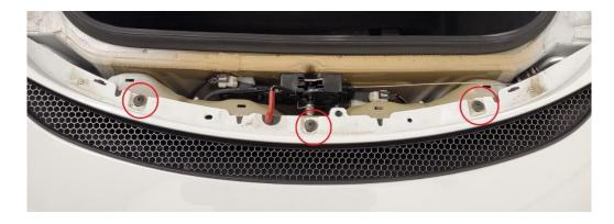
**2.8.** Using a small hook pull out the bumper release tabs on the inside of the headlight housing.
