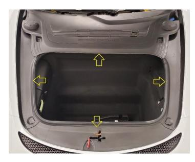
**2.7.** Remove the bumper bolts with a T30 torx socket.
