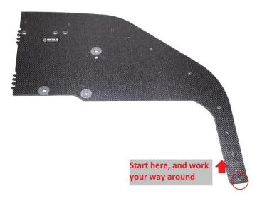
**2.44.** With all the M6 bolts started and the M4 studs lined up correctly, center the splitter, and begin tightening the M6 BHCS to 6 ft-lbs.
