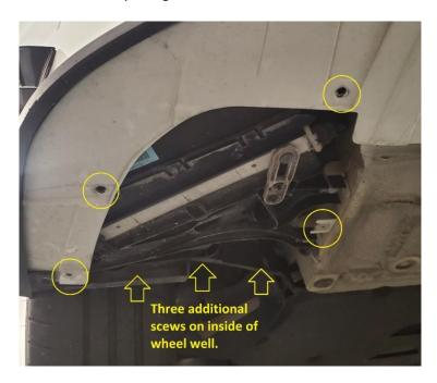
**2.12.** Remove the Torx head bolts along the bumper / fender liner edge.
