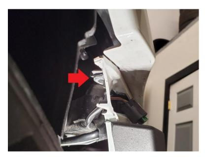
**2.14.** On both sides, disconnect the connector behind the fender liner. If you peel the liner back, the connector is about 12 inches inboard. You can also follow the harness coming from the marker light area.
