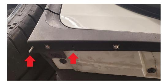
**2.42.** Bolt the splitter to the splitter brackets. Start from the center and work outward. Ensure that all of the bolts start smoothly, and that all of the m4 studs come through their corresponding holes. These are the bolts installed to the splitter in **2.40**.
