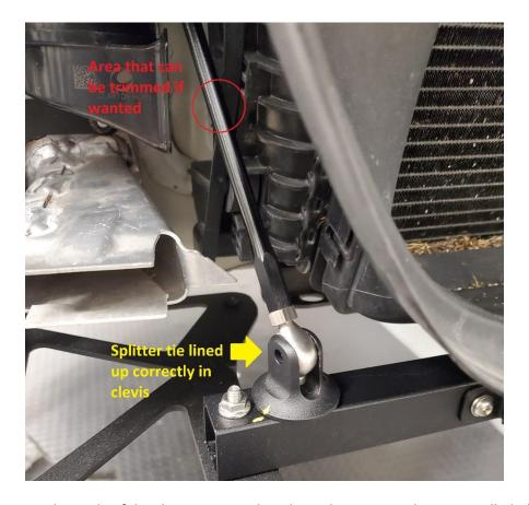
**2.33.** As the angle of the clevises cannot be adjusted once everything is installed, the crash bar should be removed at this time, and the clevises should be torqued to 6 ft-lbs. Be careful not to disturb the angle of the clevis during the removal.
