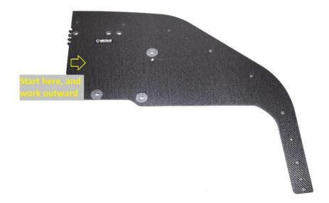
**2.43.** Working from the wheel well towards the center, begin replacing the M4 studs with 20mm long M4x.7 BHCS, and fender washers. The studs can be removed with a 2mm allen socket. The bolts can be installed with a 2.5mm allen socket. Torque to 3 ft-lbs
