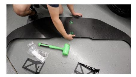
**2.4.** Next hold the splitter up to the bottom side of the bumper, and marking the holes shown in the following steps. Half of the splitter blade is shown; however, the two halves are mirrored minus the logo plate. Make sure the splitter is centered, and the rear portions are flush against the wheel well edge.
