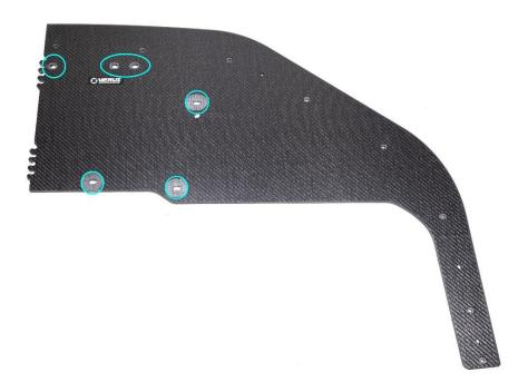
2.4.2. Next, drill the highlighted holes to 5/32" on both sides along the air dam.
