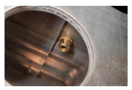
**2.23.** Install a clevis into both rivet nuts using two 25mm long low profile SHCS. Do not tighten them at this time, just snug them up so that they can still move freely. Insert the low profile SHCS from the top of the clevis. Below is an example of the orientation of the bolt and clevis. This orientation will be used for all clevises installed in this kit.
