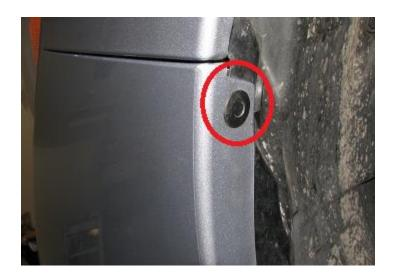
**4.4.** Moving to the top of the bumper, we need to remove the plastic rivets here as well, and the 10mm bolts scattered throughout. The 10mm are circled in yellow. The plastic rivets are circled in blue.
