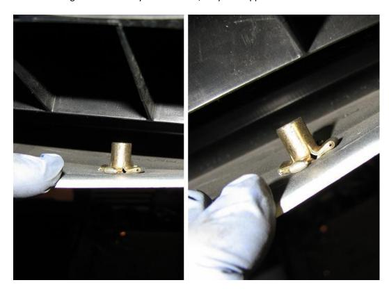
**3.12.** Below is a photo of the outside three rivet nuts installed on the car. Note how the rivet nut is above the black plastic shield.
