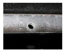
**4.11.** Using the tape measure, the hole to hole spacing should be ~20.0" as shown below. Using the same procedure (center punch, pilot hole, 1/4" hole), drill this hole out as shown below as well. **Once again note, the hole is drilled between the two spot welds (blue arrows), this is important as drilling through a spot weld is difficult.**
