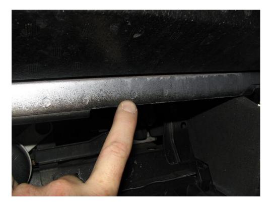
**4.8.** Using a tape measure, measure ~2" from the center strengthening rib on the crash beam (see below picture for a representation of this). Make a mark with a pencil or marker (circled in red). **Note: This should be in between the spot rivets, marked with yellow arrows in the below picture as well.**
