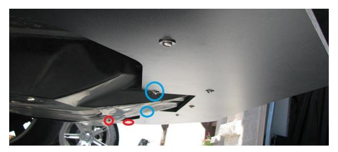
**3.18.** The next bolts to be installed are the front five units, which all need spacers/washers installed above them to be installed perfectly flat. Typically the two units circled in green, which are M6 x 1.0 x 35mm long, use the 5mm spacer above the splitter (circled in green). Hint: To slide the spacers in, pull down on the splitter and slide the spacer between the splitter and the car.
