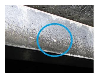
**4.10.** Using a starter drill bit or a pilot sized drill (1/8"), drill the center punched hole out. Using the 1/4" drill bit, increase the size of this hole to 1/4" as shown below.
