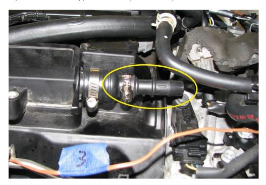
**2.15.** Before fitting the 1/2" inch hose to the engine air intake, loosen the clamps for the rubber hose of the engine air intake using a 7/32" socket and rotate rubber hose inwards as shown below. Tighten after rotating.
