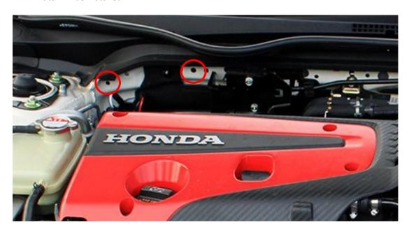
**2.6.** The M4x0.7 rivet nut will be installed in the outer hole (red) and the M5x0.8 rivet nut will be installed in the inner hole (blue).
