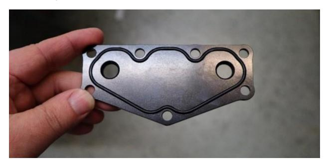
**3.1.2.** Fit the backing plate to the AOS using the four 16mm long M6 BHCS and 12mm M6 washers in the four outermost locations. Make sure the o-ring does not come unseated and get pinched. After the backing plate is installed with the four bolts and washers, install the bracket using the remaining the 16mm long M6 BHCS, and torque to 6 ft-lbs.
