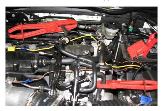
**3.4.** Remove the rear coolant hose line using hose clamp pliers or needle nose pliers.
