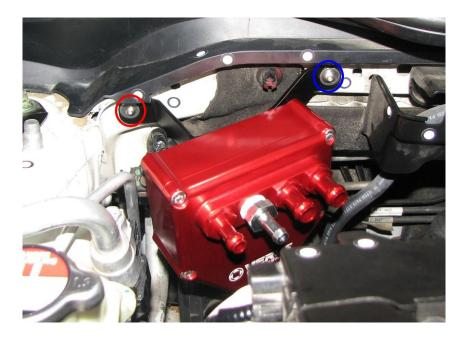
**2.19.** Using two hose line clamps, clamp the two coolant hoses that connect to the metal coolant line that is welded to the OEM crankcase ventilation pipe.
