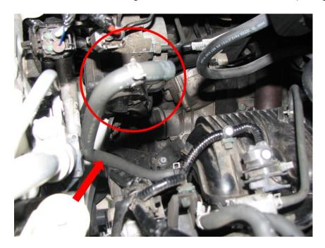
2.9. Loosen the clamps for the crankcase ventilation system. Honda uses security clamps (yellow). There are several methods of removing these. You can grip the "head" with some pliers or cut a slit in the head using a Dremel and then use a flathead screwdriver. If that doesn't work, cut the clamp entirely with extra caution not to cause any damage. We supply replacement clamps (red) and recommend using them over the OEM clamps. We only need to remove the red clamps circled below for the install.
