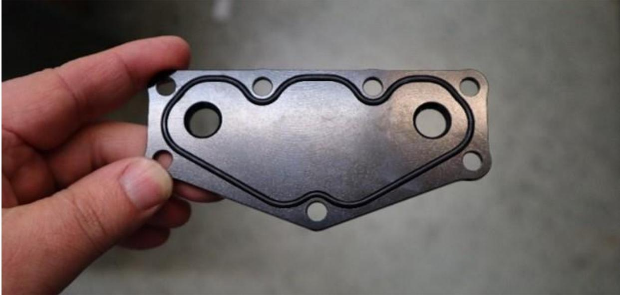
**3.1.2.** Fit the backing plate to the AOS using the four 16mm long M6 BHCS and 12mm M6 washers in the four outermost locations. Make sure the o-ring does not come unseated and get pinched. After the backing plate is installed with the four bolts and washers, install the bracket using the remaining the 16mm long M6 BHCS, and torque to 6 ft-lbs.
