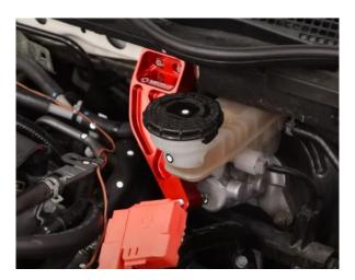
**2.10.** Now it is time to adjust the adjuster bolt and install the foot. To do so, unthread the adjuster bolt until it is nearly touching the BMC and then slide the foot between the BMC and the adjuster bolt. Tighten by hand until the foot stays in place. Ensure the foot is centered on the master cylinder brace and then loosen the adjuster to add some compression to the master cylinder. Do not go overboard, a little resistance is good.
