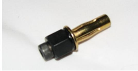
**2.6.** Using the 9/16" wrench and the 3mm allen wrench, hold the nut steady and tighten the allen bolt. You will have some initial resistance, then the rivet nut will begin to pull tighter on the material.
