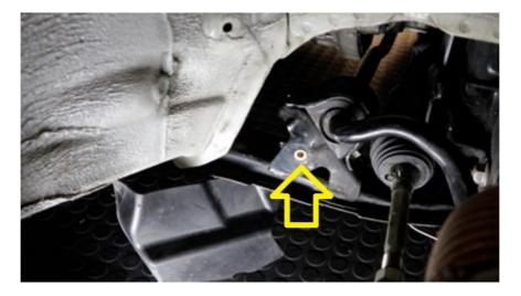
**2.6.** To properly install the rivet nut, you will want to thread the rivet nut onto the tool as shown below, and place the rivet nut into the hole.
