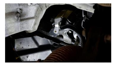
**2.10.** Reinstall the factory plastic shield reusing the pop rivet in the upper location only.
