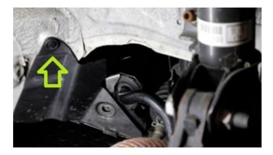
**2.11.** Grab your M5 SHCS and washer and install as shown below. Using your 4mm allen socket or key, torque to 5-6 ft-lbs.
