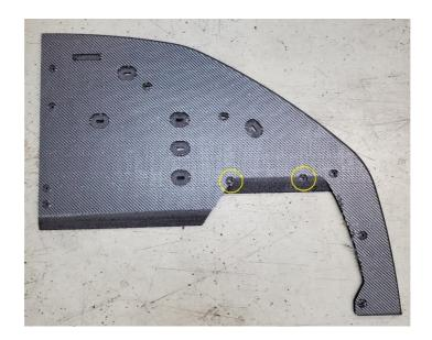
**2.29.** Once all of the bolts are started, tighten the M6 BHCS to 6 ft-lbs, and the THCS to 4 ft-lbs. moving from the center to the outside is recommended.
