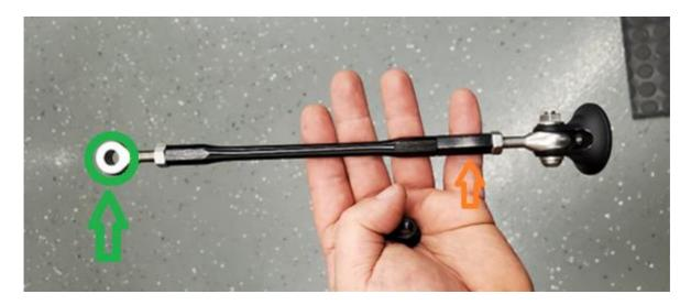
**2.20.** Reusing the 13mm nut from the tension cable, bolt the support rod to the crash bar, and use a 12mm M6 BHCS with 12mm washer to bolt the clevis to the cross brace. Torque the M6 BHCS to 6 ft-lbs, and the OEM 13mm nut to 13 ft-lbs. The support rod should be passing through the radiator duct cut-outs as shown below.
