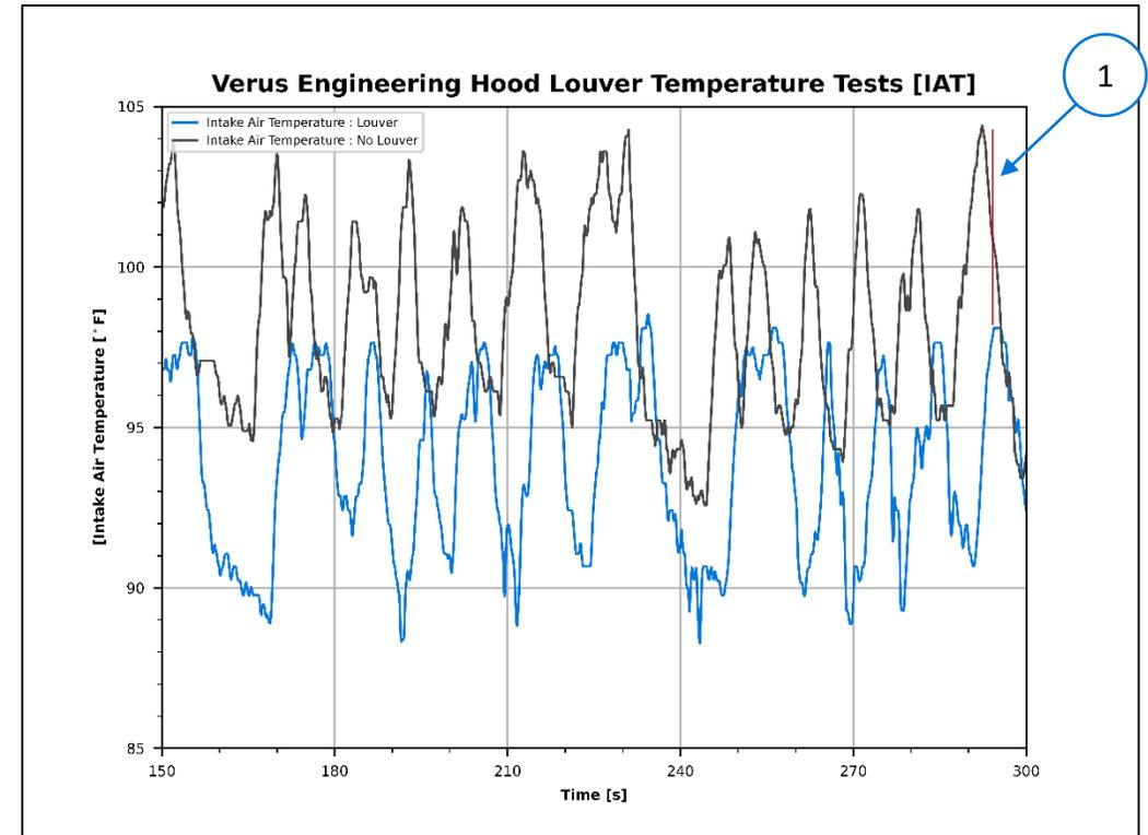
The temperature just after the airbox [Intake Air Temperature] is around 4-6 degrees Fahrenheit **lower** with the Verus Engineering Hood Louver. The hood louver helps evacuate the higher temperatures in the engine bay which helps drop the intake air temperature. Lowering the IAT's can increase horsepower output.
