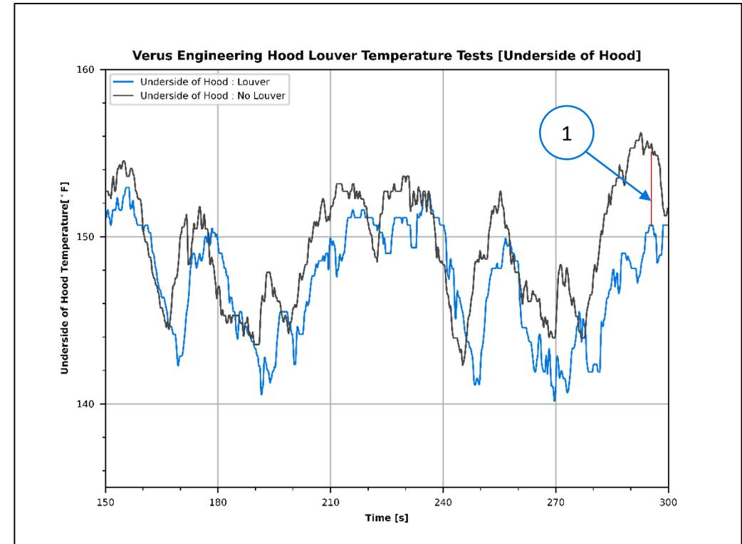
The temperature under the hood is around 3-5 degrees Fahrenheit lower with the Verus Engineering Hood Louver. The hood louver helps keep the engine bay cooler by evacuating the hot air from the engine bay.
