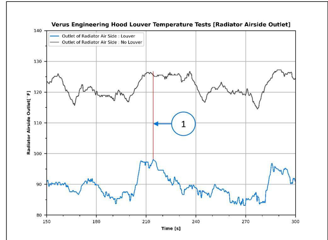
The temperature behind the radiator [Outlet of Radiator Air Side] is around 25 degrees Fahrenheit lower with the Verus Engineering Hood Louver. The hood louver helps evacuate the hot air that has passed through the radiator.
