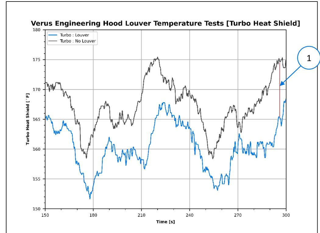
The temperature around the turbo heat shield and turbo is around 6-8 degrees Fahrenheit lower with the Verus Engineering Hood Louver. The hood louver helps evacuate the higher temperatures in the engine bay which helps evacuate the heat produced by the turbocharger and manifold.
