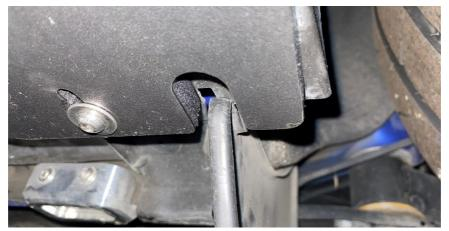
**2.5.** Holding the side splitter still, mark each slot with a paint marker or Sharpie. Having a second set of hands to hold the side splitter stationary is beneficial here. Ensure both ends of the side splitter sit flush with the front and rear of the factory side skirt as shown below.
